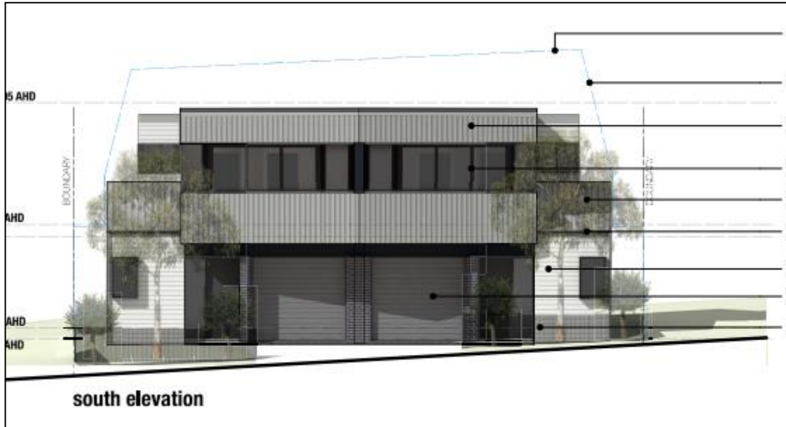
Figure 9: Proposed development viewed from Elder Street with the NDCP 2012 building envelope identified by blue dashed outline.
