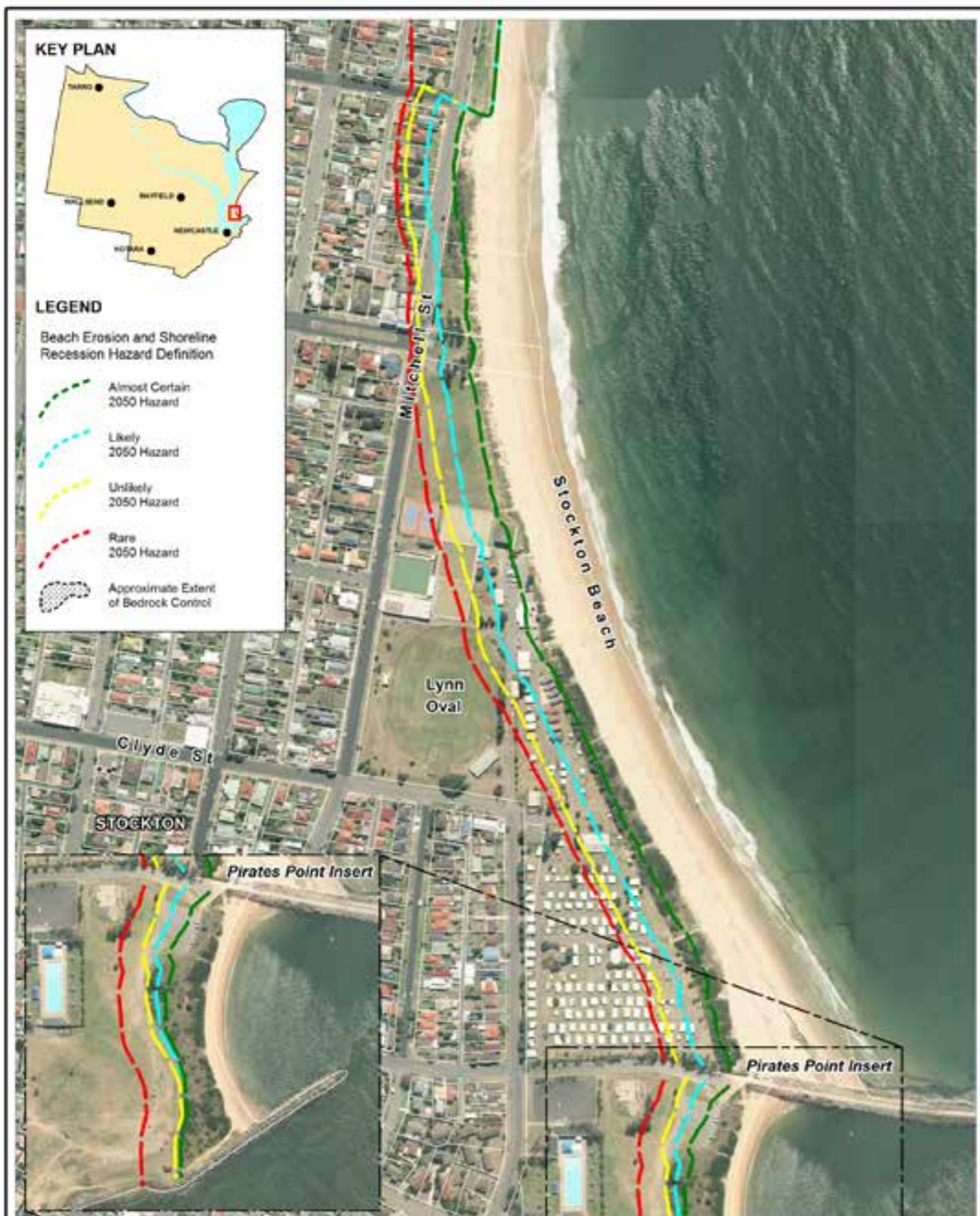
Title: Erosion and Recession Hazard Definition 2050 Planning Horizon - Stockton South Figure: B-4 Rev: A BMT WBM endeavours to ensure that the information provided in this map is correct at the time of publication. BMT WBM does not warrant, guarantee or make representations regarding the currency and accuracy of information contained in this map. 0 100 200m Approx. Scale BMT WBM www.bmtwbm.com.au Filepath : K:\N2051_NewcastleCoastalHazards&Management\MI\Workspaces\DRG_204_111025_Drawing_B-4.WOR
