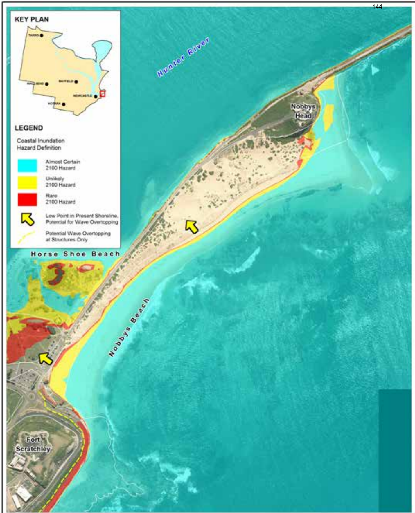
Title: Coastal Inundation Hazard Definition 2100 Planning Horizon - Nobbys Beach Figure: F-5 Rev: A BMT WBM endeavours to ensure that the information provided in this map is correct at the time of publication. BMT WBM does not warrant, guarantee or make representations regarding the currency and accuracy of information contained in this map. Approx. Scale www.bmtwbm.com.au Filepath : K:\N2051_NewcastleCoastalHazards&Management\MI\Workspaces\DRG_605_111025_Drawing_F-5.WOR
