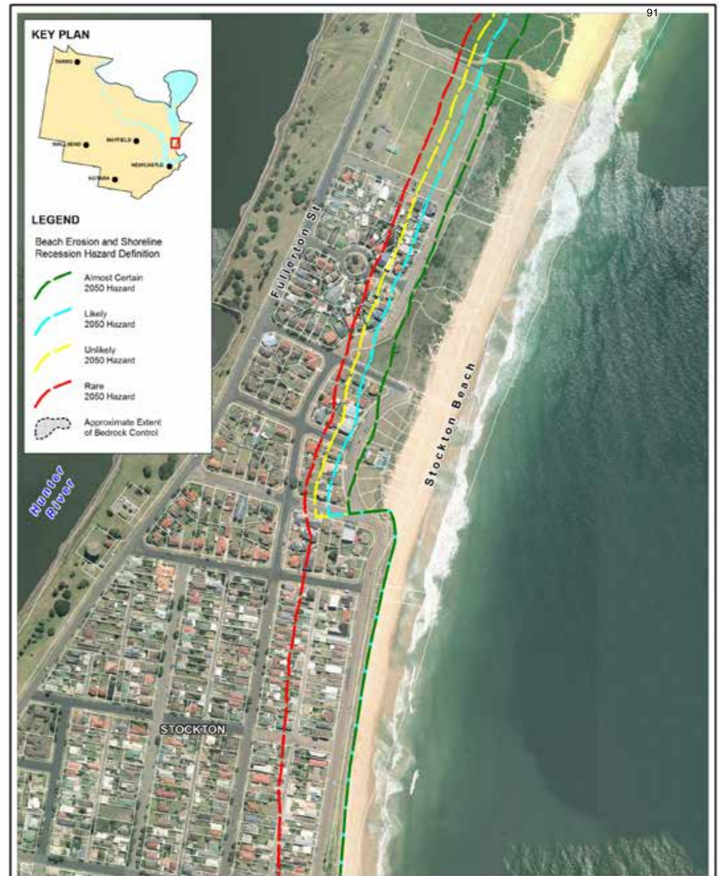
Title: Erosion and Recession Hazard Definition 2050 Planning Horizon - Stockton North Figure: B-3 Rev: A BMT WEM endeavours to ensure that the information provided in this map is correct at the time of publication. BMT WEM does not warrant, guarantee or make representations regarding the currency and accuracy of information contained in this map. www.bmtwbm.com.au Filepath : K:\N2051_NewcastleCoastalHazards&Management\MI\Workspaces\DRG_203_111025_Drawing_B-3.WDR
