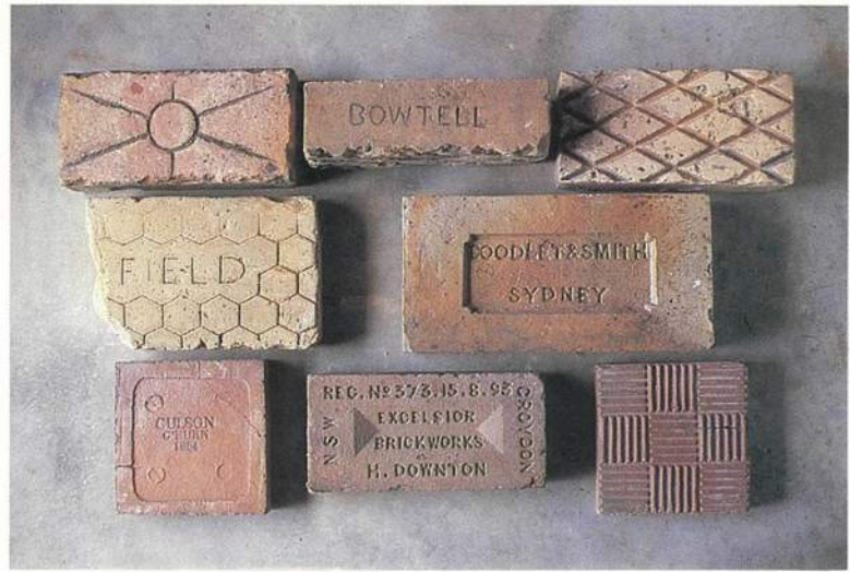
EXAMPLES OF PAVING BRICKS USED IN NEWCASTLE AND PARTICULARLY IN WICKHAM BRICK 1 & 3 WITH ITS DIAMOND PATTERNS SERVED AS INSPIRATION FOR THE DESIGN OF PRECAST CONCRETE WALL PATTERN (BOOK SOURCE: "AND SO WE GRAFT FROM SIX TO SIX, THE BRICKMAKERS OF NEW SOUTH WALES" BYWARWICK GEMMELL)
