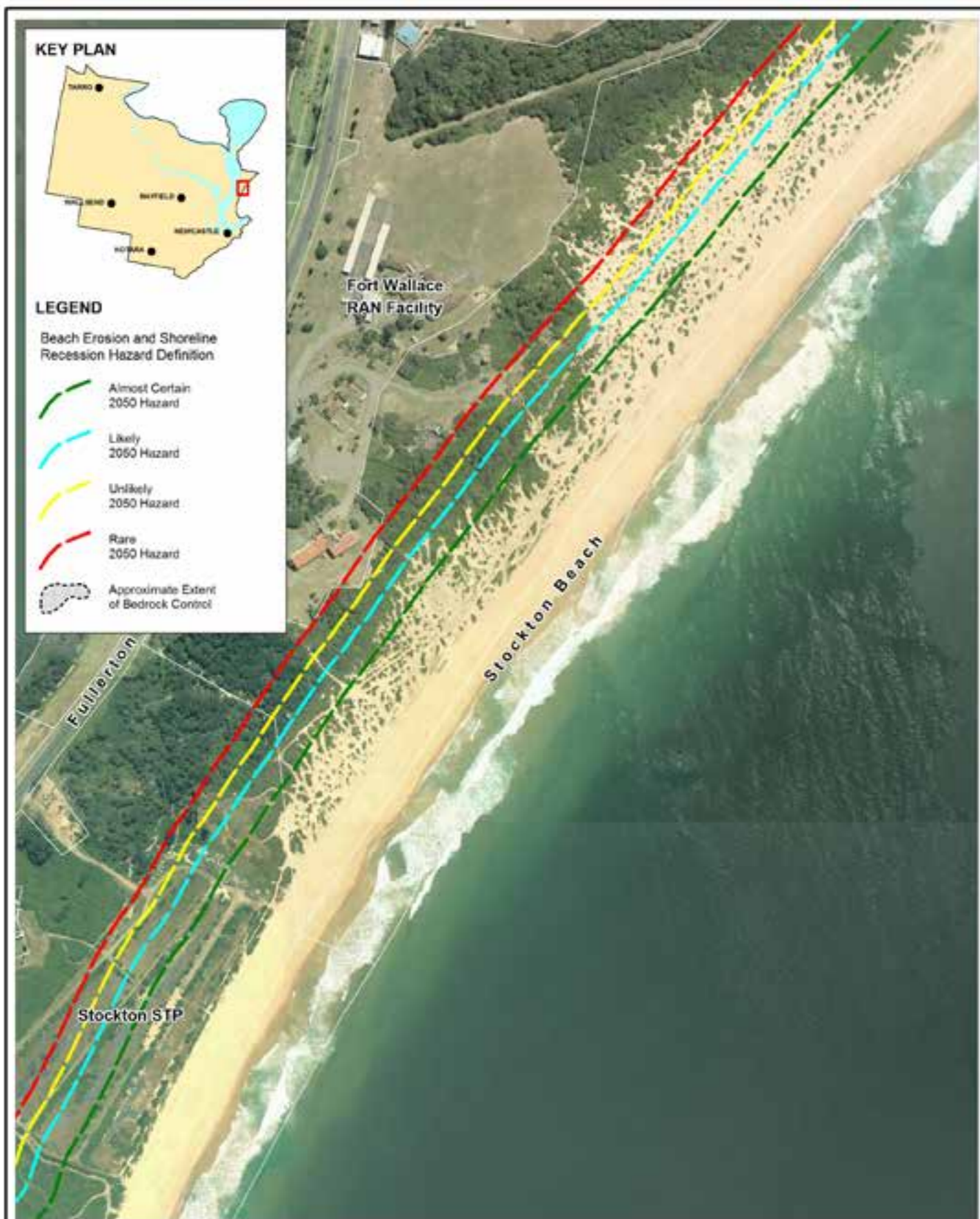
Title: Erosion and Recession Hazard Definition 2050 Planning Horizon - Fort Wallace Figure: B-2 Rev: A BMT WEM endeavours to ensure that the information provided in this map is correct at the time of publication. BMT WEM does not warrant, guarantee or make representations regarding the currency and accuracy of information contained in this map. Filepath : K:\N2051_NewcastleCoastalHazards&Management\M\Workspaces\DRG_202_111025_Drawing_B-2.WDR
