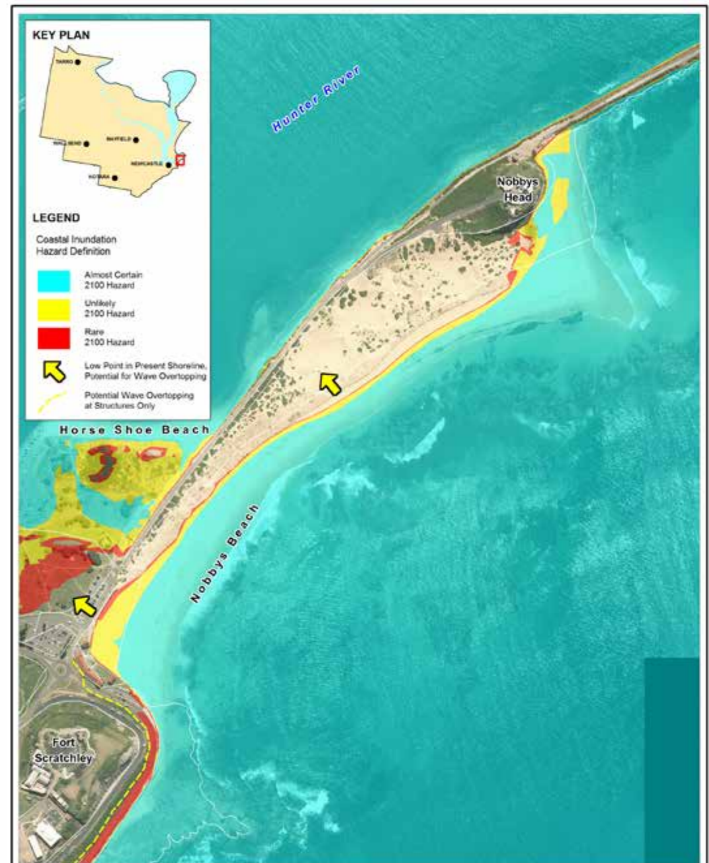
Title: Coastal Inundation Hazard Definition 2100 Planning Horizon - Nobbys Beach Figure: F-5 Rev: A BMT WBM endeavours to ensure that the information provided in this map is correct at the time of publication. BMT WBM does not warrant, guarantee or make representations regarding the currency and accuracy of information contained in this map. N 0 100 200m Approx. Scale BMT WBM www.bmtwbm.com.au Filepath: K:\N2051_NewcastleCoastalHazards&Management\MI\Workspaces\DRG_605_111025_Drawing_F-5.WOR
