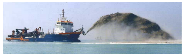
Trailing suction hopper dredger pumping at least 50m from the bow
