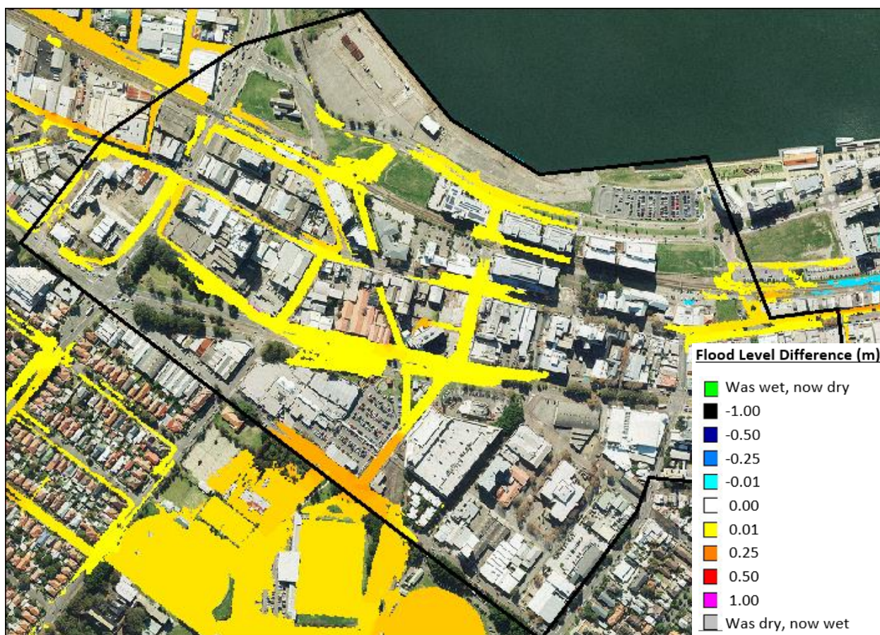
Plate 11 1% AEP flood level difference map after filling of all potentially developable land
