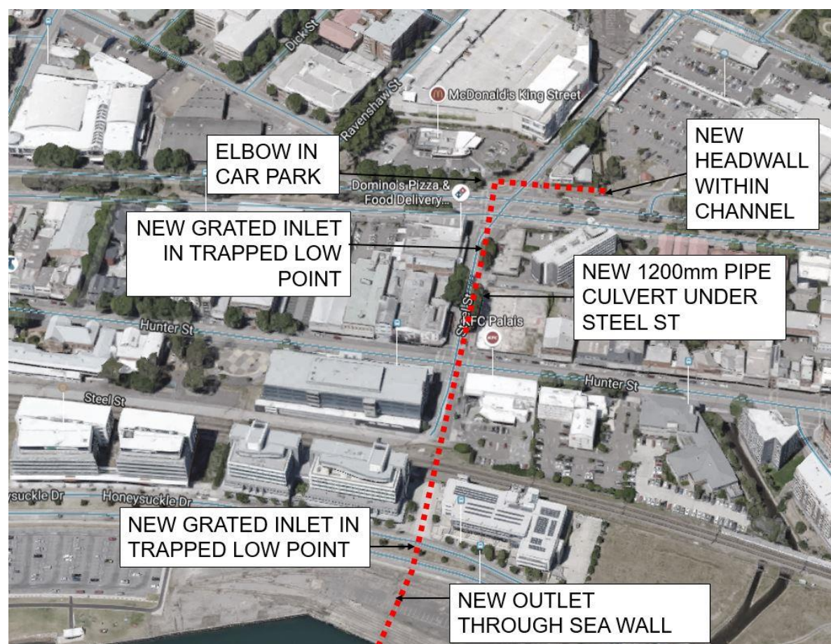
Plate 19 Proposed alignment of new culvert along Steel Street looking south from Newcastle Harbour
