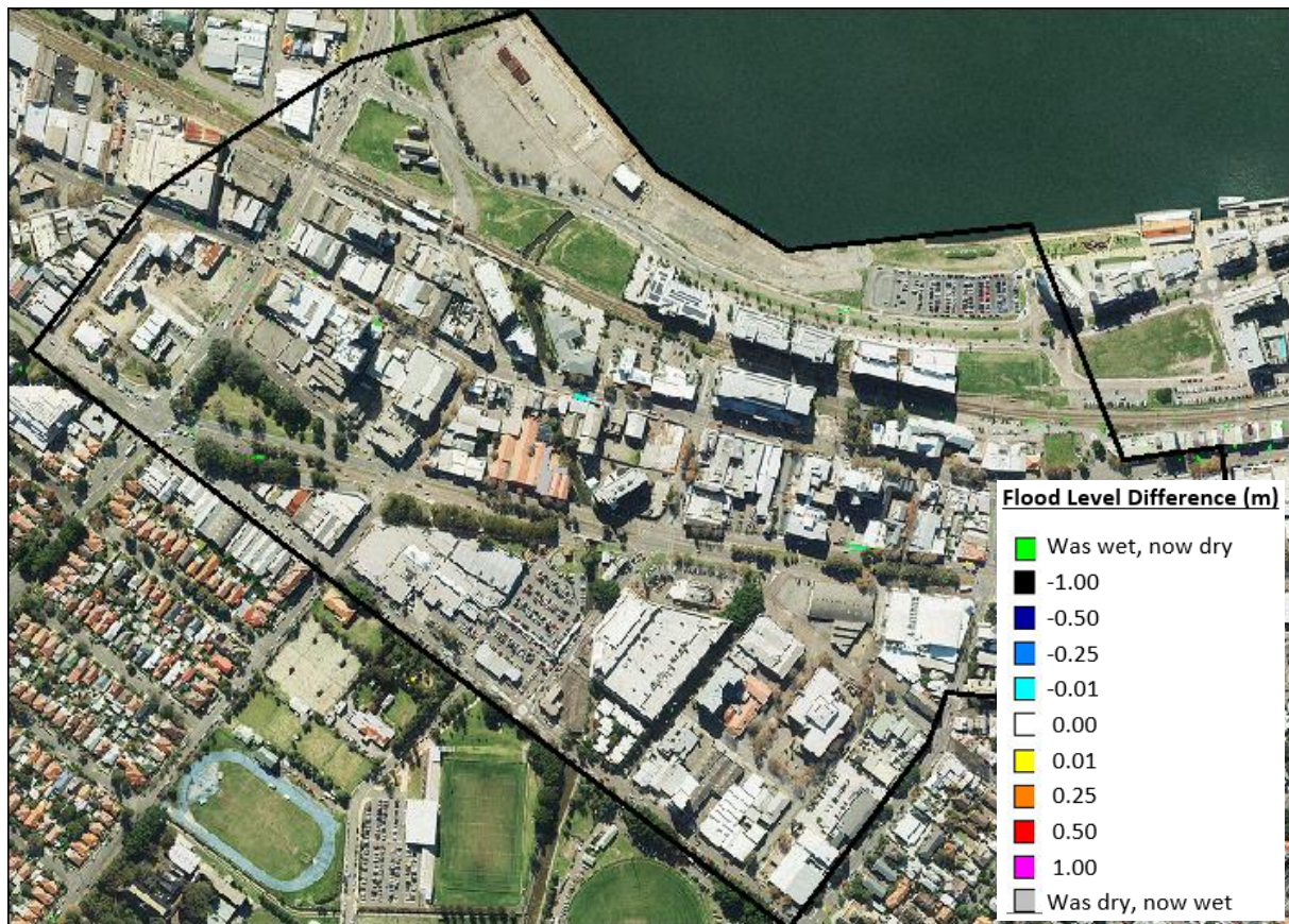
Plate 9 1% AEP flood level difference map with no blockage
