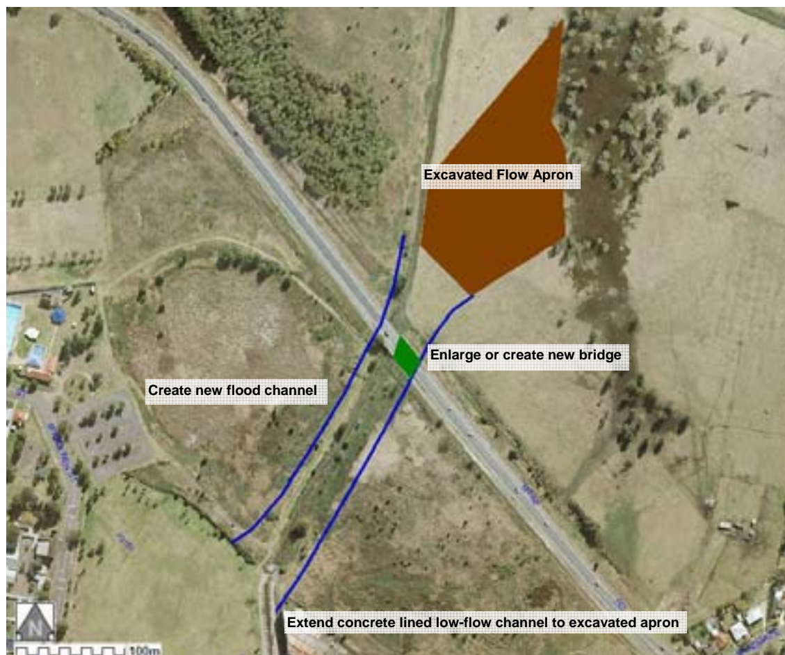
Figure 4 - Downstream Channel Schematic Configuration
