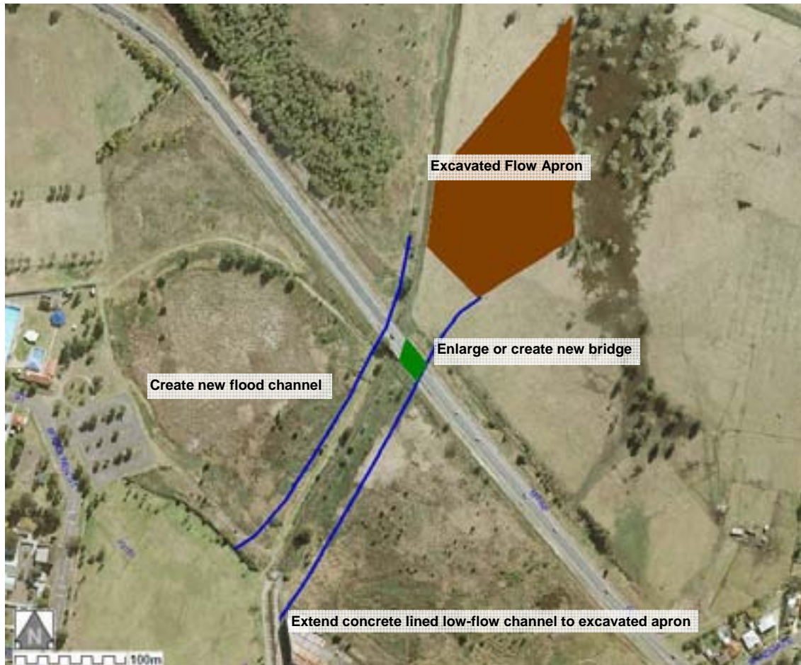
Figure 19 - Downstream Channel Schematic Configuration
