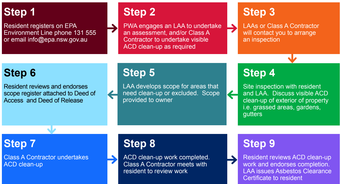
Figure 8 – Wickham Wool Store Fire ACD Clean-up Flowchart for Properties Assessed as Having Level 1 or 2 Impact
