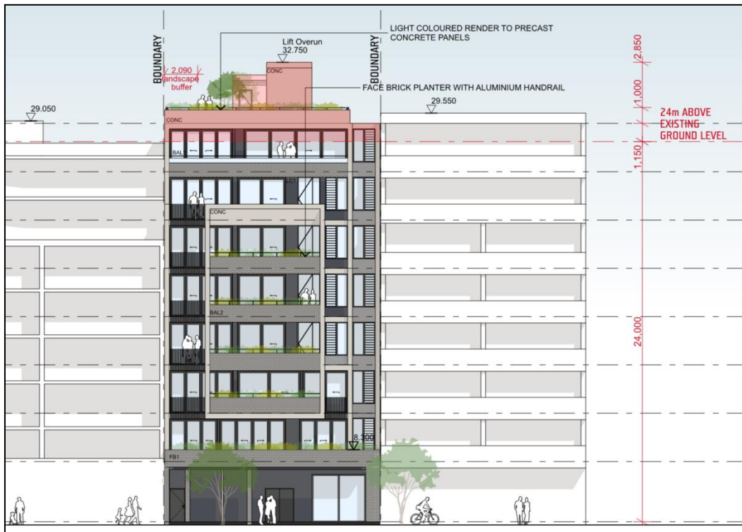
Figure 1: Extract of South Elevation (Parry Street) – extent of height exceedance shown in red
