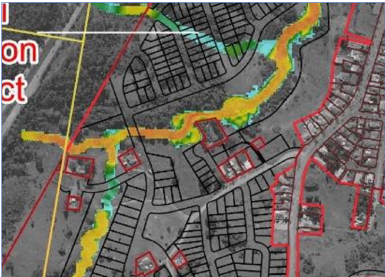
Figure 36 – Existing Peak Flood Depth 1%AEP with 1%AEP Tailwater – Vicinity of existing Railway Street properties (Source BMT Report, Figure 3-8)
