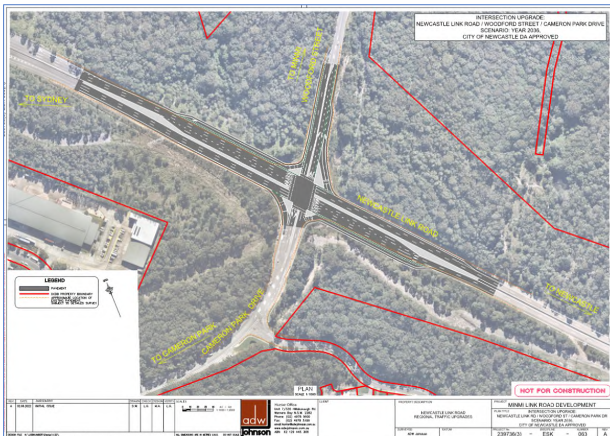
FIGURE 26 – Conceptual Plan of Road Upgrade – Intersection Newcastle Link Road and Woodford St - 2036 (Source – Attachment 7 – State Road Upgrades (CN DA), Sht 8)
