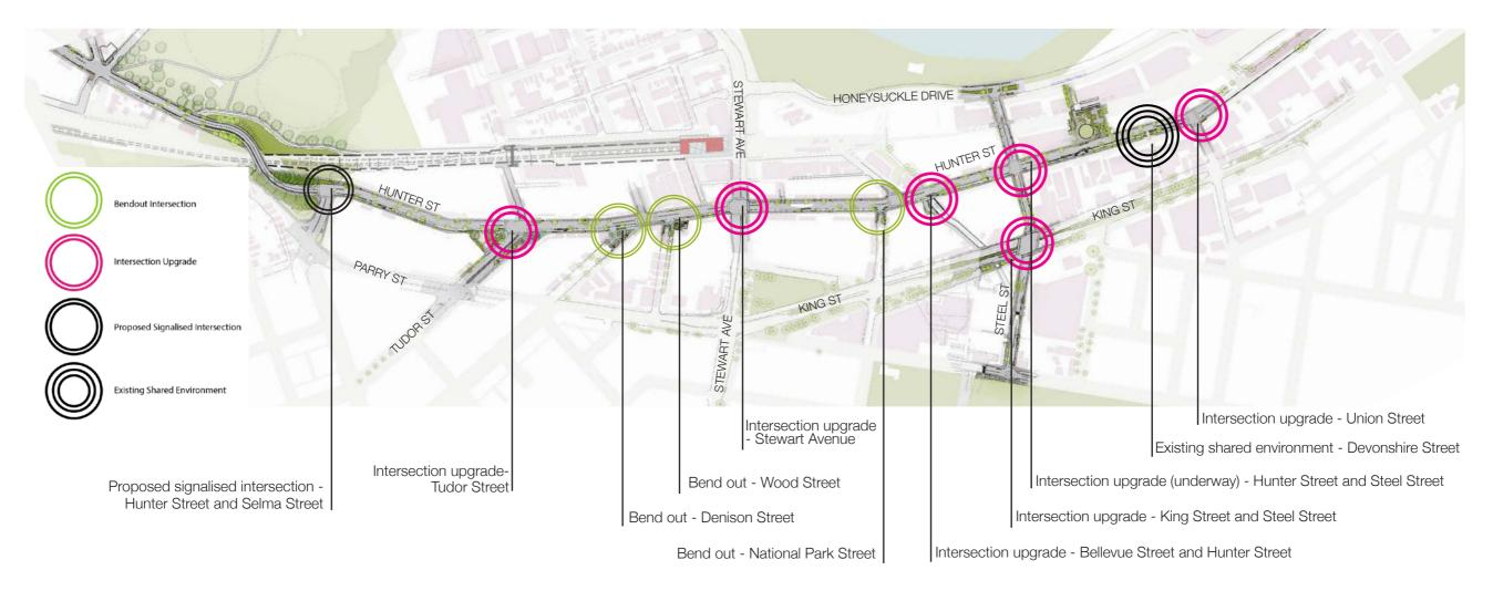
The separated cycleway is a significant modification to the current function of the street. In effect, the existing road easement will now accommodate two parallel two-way systems - the vehicle road and the bicycle path (City of Sydney, 2008).
