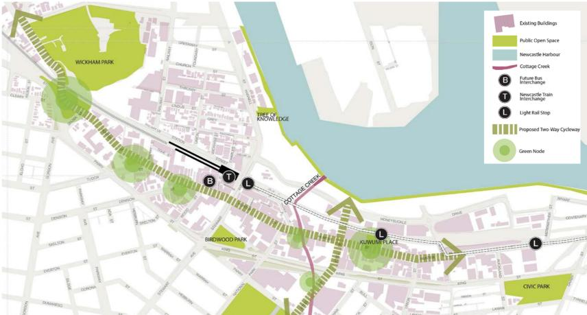
Key links, green nodes and gateways along proposed two-way separated cycleway
