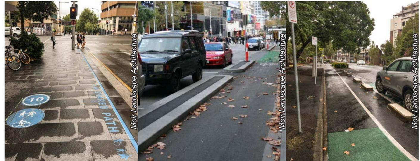
Precedent imagery of a shared path, a double step two-way separated cycleway and a median barrier two-way separated cycleway, currently used in Sydney
