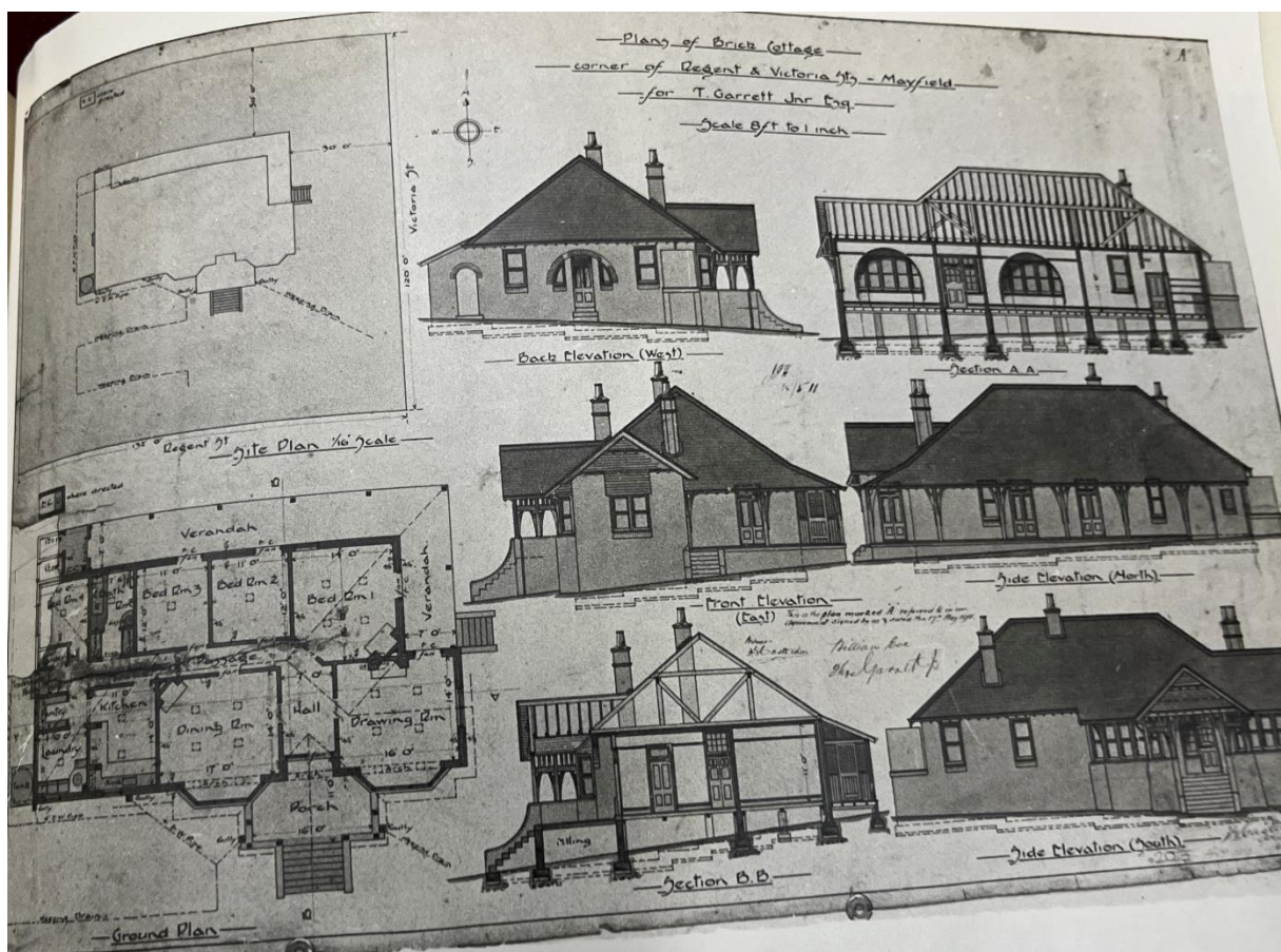
Figure 9: Architectural Drawings for 22 Victoria Street Mayfield Source: "The Work of F.G. Castleden, 1907–1919: An Architectural Thesis" John Sara.
