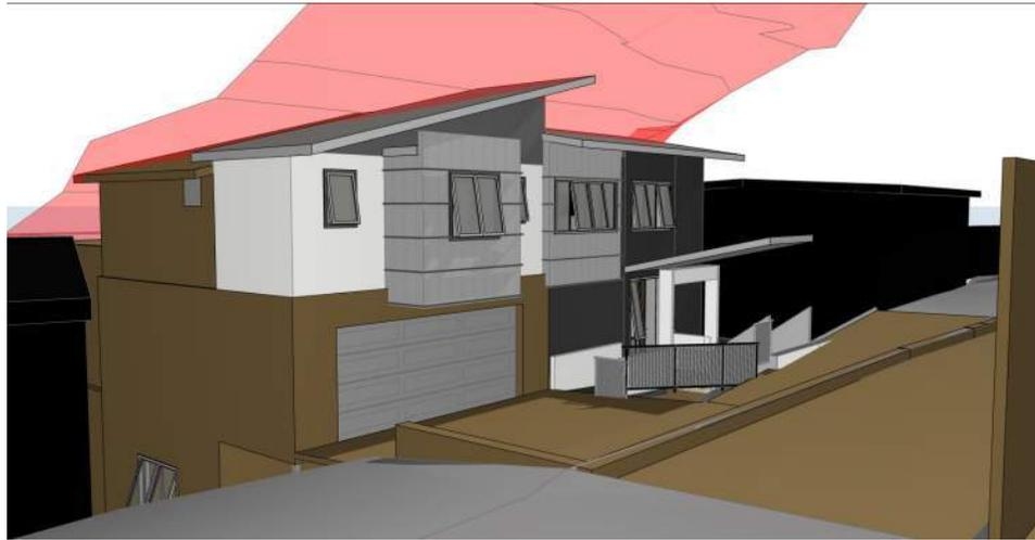
Figure 6 - Computer generated 3D image showing the CoN maximum building height control as viewed from the rear.
