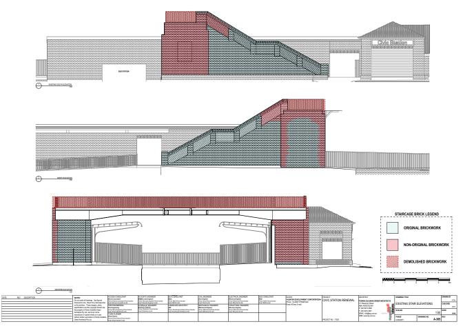
Figure 163: Civic Railway Station, Existing Footbridge Elevations, showing extent of original brickwork.
