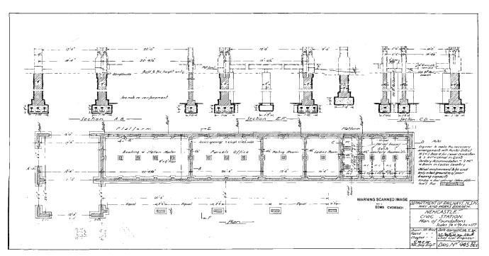
Figure 22: 1935 - Newcastle, Proposed Civic Station, Plan of Foundations, Department of Railways NSW Way and Works Branch. Dwg No. 945-27/065.
