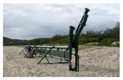
Figure 4: Example submerged sand extraction unit
