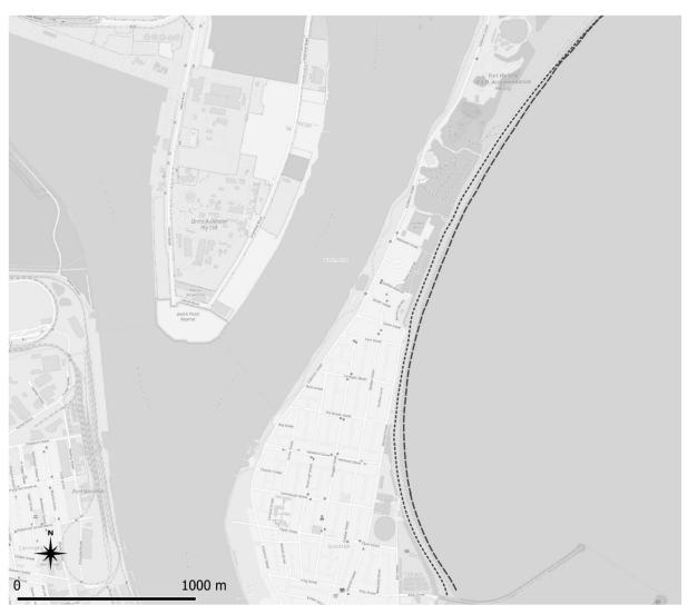
Figure 12: Mean sea level (0m AHD) shorelines from 2018 (inner) and 1994 (outer) showing realignment of the southern embayment.
