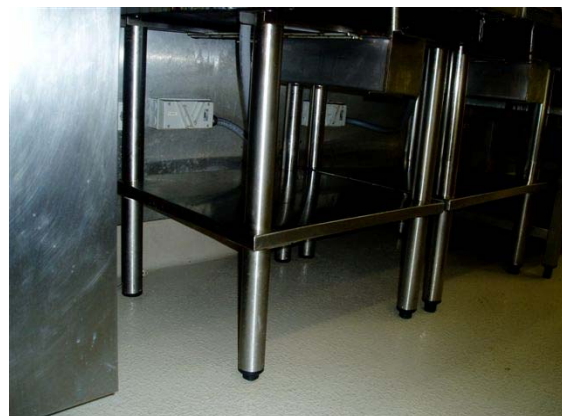
Picture 14 &15: Equipment elevated 150mm to permit cleaning underneath.
