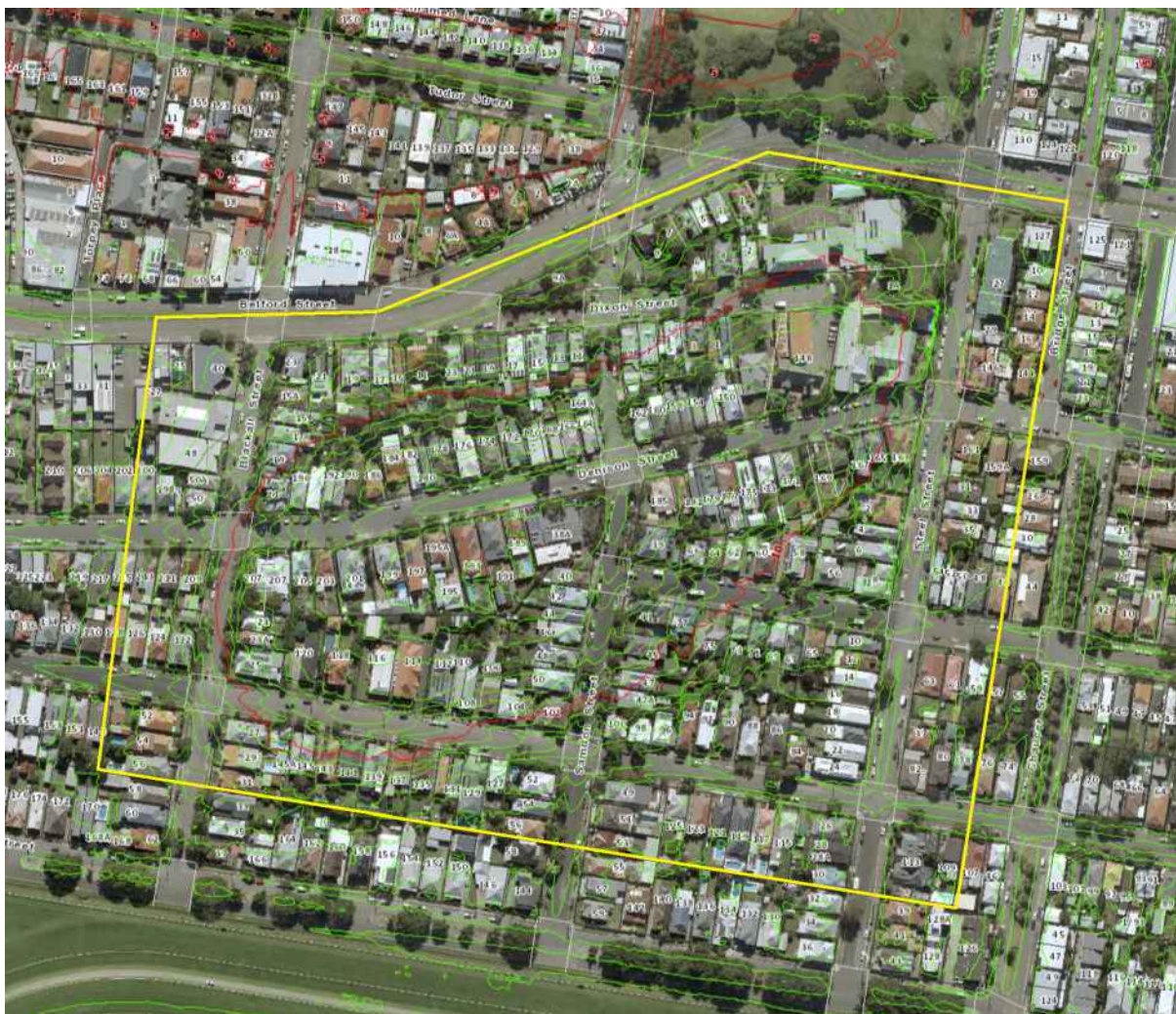
Figure 19: Topographic map of the Cameron's Hill study area. Yellow border approximates the Cameron's Hill study area. Green contour lines are at 0.5m intervals. Red contour line is 10m. (Source: CN, 2024)
