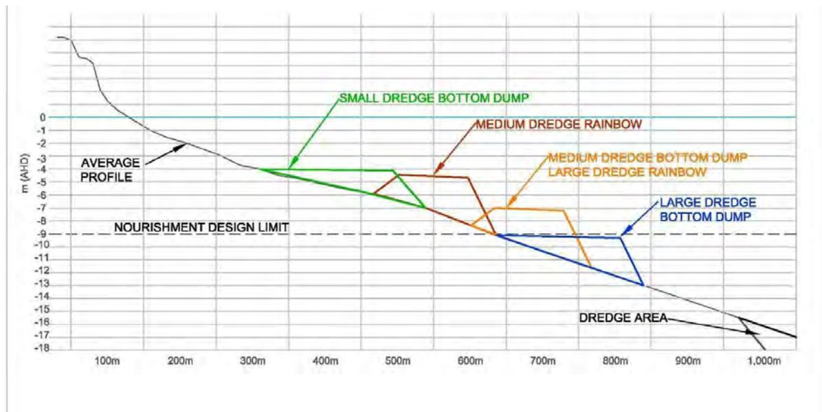
**Figure 4.10: Placement Depths for Various Dredger Sizes (Corbett and Salyer, 2014)**
