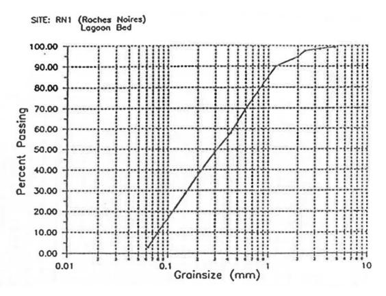
Figure 3.2: Example Sand Grading Curve
