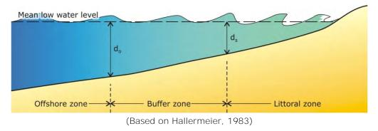
Figure 2.3: Concept of Closure Depth
