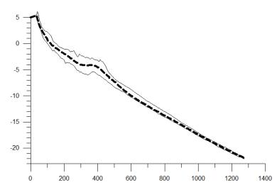
Figure 2.2: Envelope of surveyed cross-shore (ETA63) profiles of Surfers Paradise (1976 to 1997)
