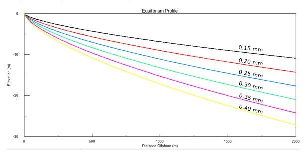
Figure 3.3: Equilibrium Profile for Various Sand Grain Sizes
