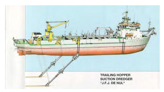
Figure 4.5: Trailing Suction Hopper Dredger (Jan de Nul Group)
