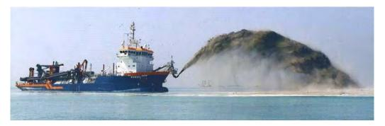
Figure 4.7: Trailing Suction Hopper Dredger Rainbowing (Van Oord Australia)
