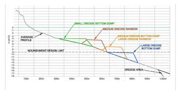
Figure 4.10: Placement Depths for Various Dredger Sizes (Corbett and Salyer, 2014)
