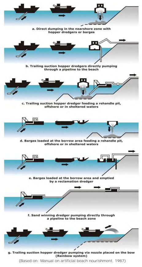
Figure 4.4: Some Methods of Undertaking Dredger Nourishment
