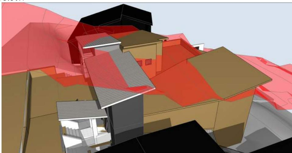
Figure 1 -Computer generated 3D image aerial view showing the CoN maximum building height control as a three dimensional plane in red at a height of 8.5m above the natural ground line. The existing elements are shown in dark beige colour.The adjacent dwellings are shown in black.
