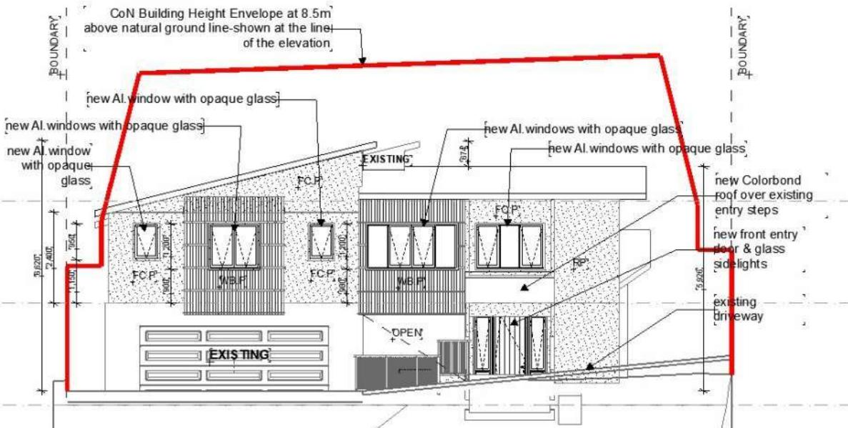
Figure 20: South Elevation noting the proposal in regard to the CoN Building Envelope and the proposed height of the roof over the new Hallway/Lift.
