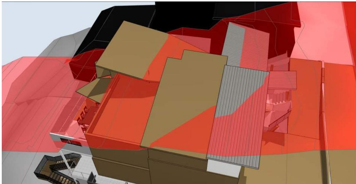
Figure 5 - Computer generated 3D image showing the CoN maximum building height control as a three dimensional plane in red at a height of 8.5m above the natural ground line as viewed from the west. The existing elements are shown in dark beige colour. The adjacent dwellings are shown in black.
