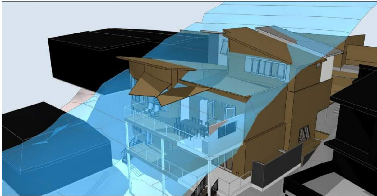
Figure 13 - Computer generated 3D image showing the CoN maximum building height control as a three dimensional plane in blue at a height of 9m above the natural ground line as viewed from above. The existing elements are shown in dark beige colour. The adjacent dwellings are shown in black.
