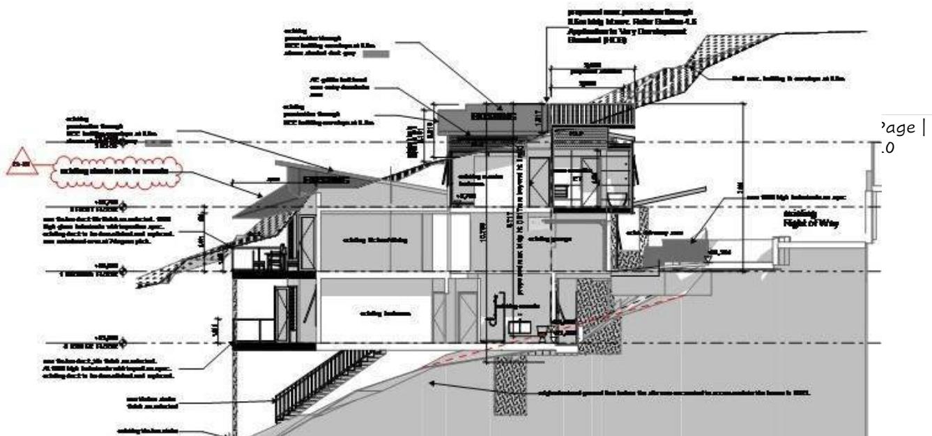
Figure 10 - Computer generated Sectional image showing the CoN maximum building height control as a three dimensional plane at a height of 8.5m above the natural ground line .
