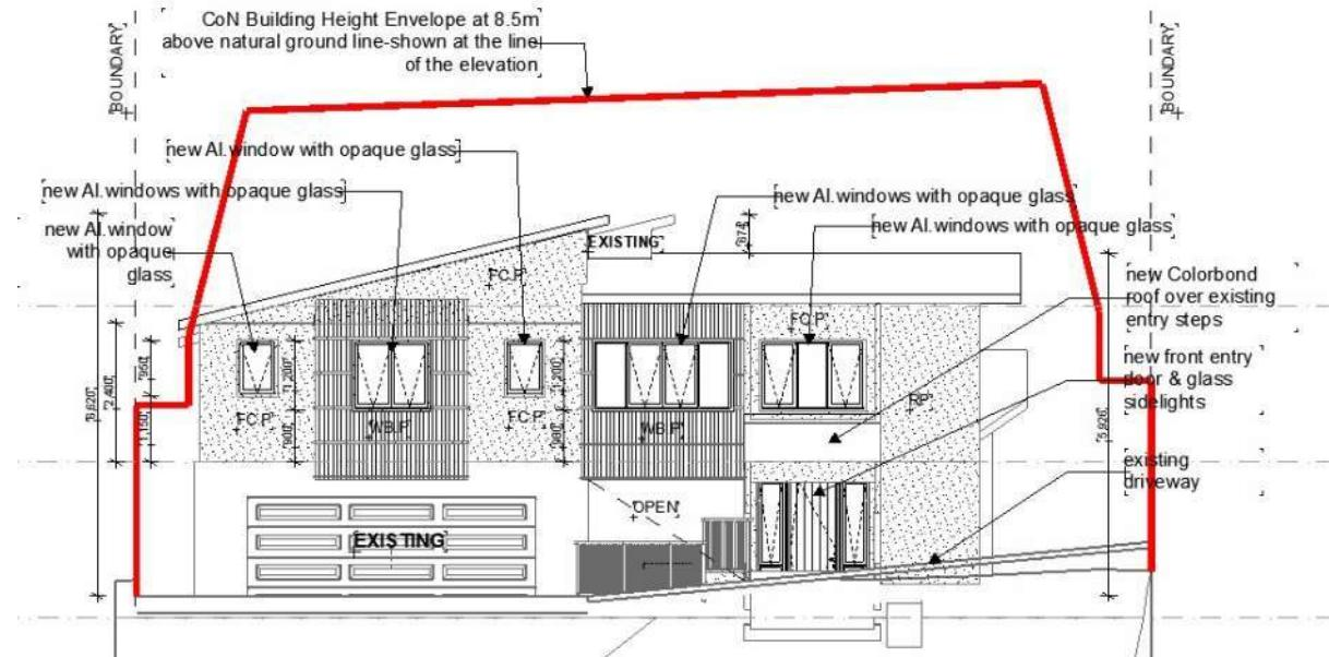
Figure 16: South Elevation showing the compliance of the addition in relation to the CoN Building Envelope.
