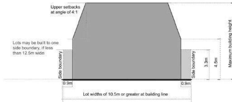
Figure 15-CoN DCP 3.02.04 showing the relevant building envelope with the maximum height shown as the top of the envelope.
