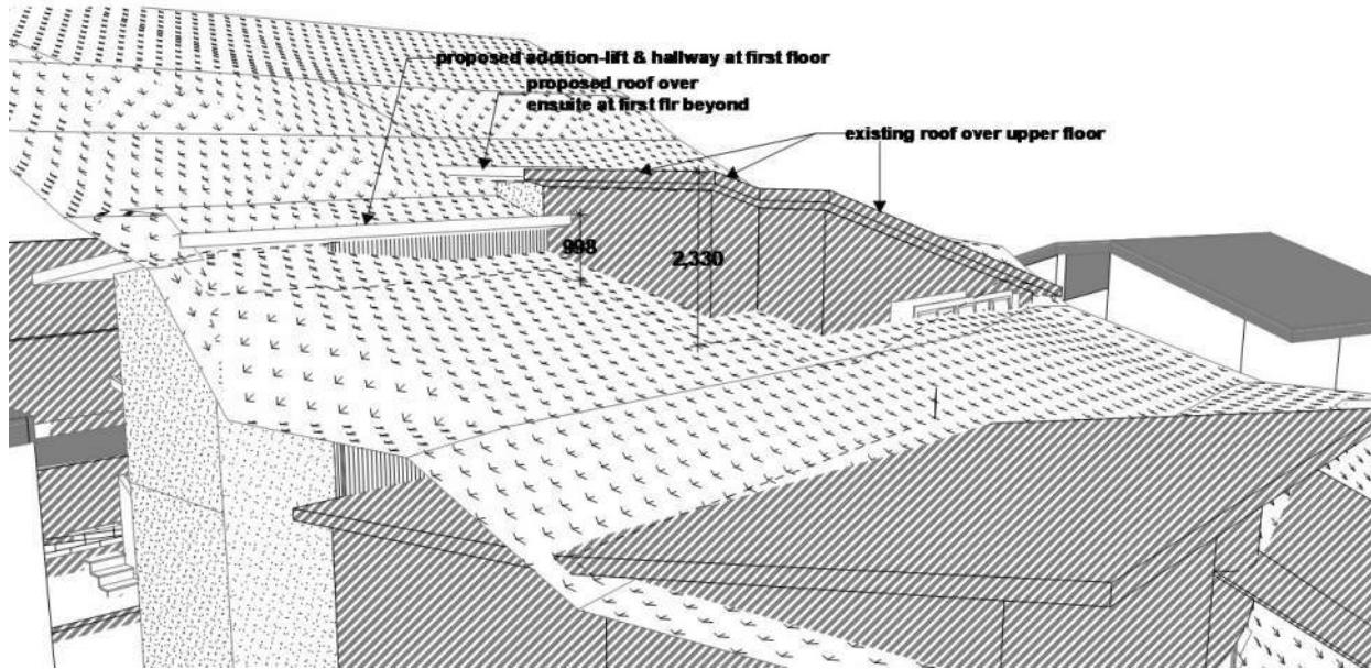
Figure 7 - Computer generated dimensioned 3D image showing the CoN maximum building height at a height of 8.5m above the natural ground line as viewed from the north-existing walls & roofs are shown in dark hatching. Dimensions shown relate to height of elements above building envelope at that point.
