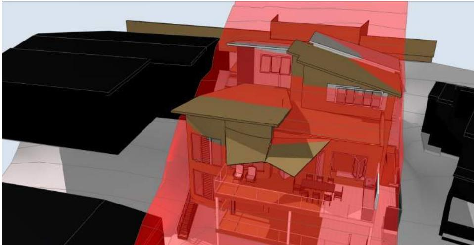
Figure 2 - Computer generated 3D image showing the CoN maximum building height control as a three dimensional plane in red at a height of 8.5m above the natural ground line. The existing elements are shown in dark beige colour. The adjacent dwellings are shown in black.
