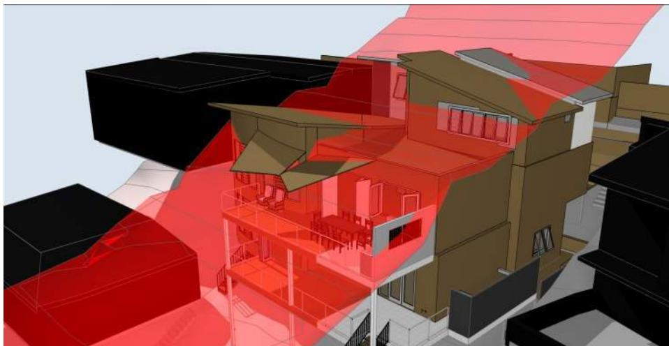
Figure 3 - Computer generated 3D image showing the CoN maximum building height control as a three dimensional plane in red at a height of 8.5m above the natural ground line as viewed from the east. The existing elements are shown in dark beige colour. The adjacent dwellings are shown in black.
