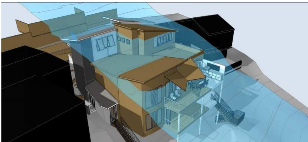
Figure 14 - Computer generated 3D image showing the CoN maximum building height control as a three dimensional plane in blue at a height of 9m above the natural ground line as viewed from the rear. The existing elements are shown in dark beige colour. The adjacent dwellings are shown in black.
