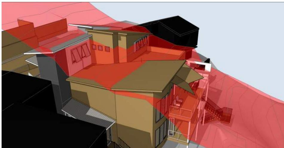
Figure 4 - Computer generated 3D image showing the CoN maximum building height control as a three dimensional plane in red at a height of 8.5m above the natural ground line as viewed from the north. The existing elements are shown in dark beige colour. The adjacent dwellings are shown in black.
