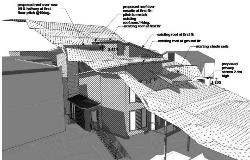
Figure 9 - Computer generated dimensioned 3D image showing the CoN maximum building height control as a three dimensional plane at a height of 8.5m above the natural ground line as viewed from the south. -
