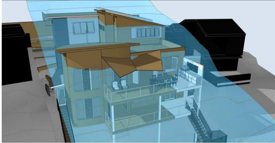
Figure 11 - Computer generated 3D image showing the CoN maximum building height control as a three dimensional plane in blue at a height of 9m above the natural ground line as viewed from above. The existing elements are shown in dark beige colour. The adjacent dwellings are shown in black.
