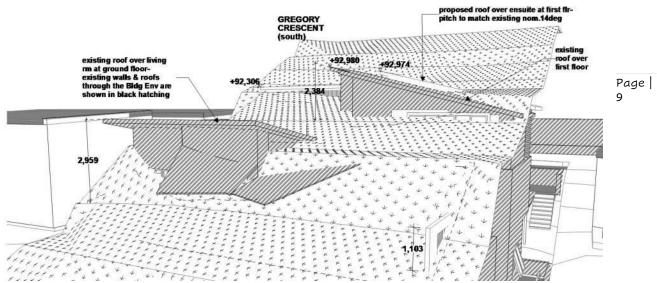
Figure 8 - Computer generated dimensioned 3D image showing the CoN maximum building height control as a three dimensional plane at a height of 8.5m above the natural ground line as viewed from above. -the existing walls & roofs are shown in dark hatching. Dimensions shown relate to height above the Building Envelope at that point.
