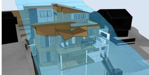
Figure 11 - Computer generated 3D image showing the CoN maximum building height control as a three dimensional plane in blue at a height of **9m** above the natural ground line as viewed from above. The existing elements are shown in dark beige colour. The adjacent dwellings are shown in black.
