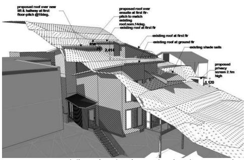
Figure 9 - Computer generated dimensioned 3D image showing the CoN maximum building height control as a three dimensional plane at a height of 8.5m above the natural ground line as viewed from the south. -
