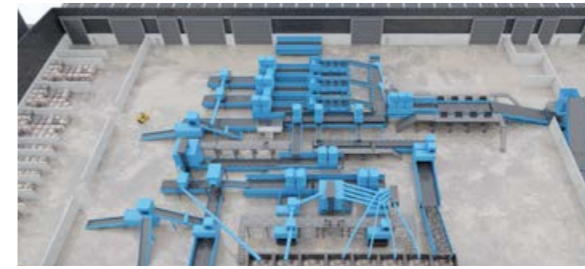
Layout of a Material Recovery Facility: A network of conveyors move the mixed recyclables through a series of equipment that sort the mixed recyclables into individual material streams.
