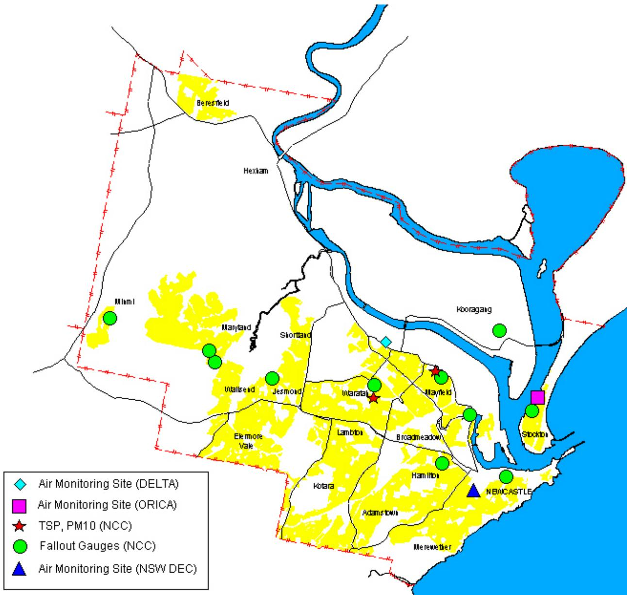
Figure 14 Air Monitoring Station Locations
