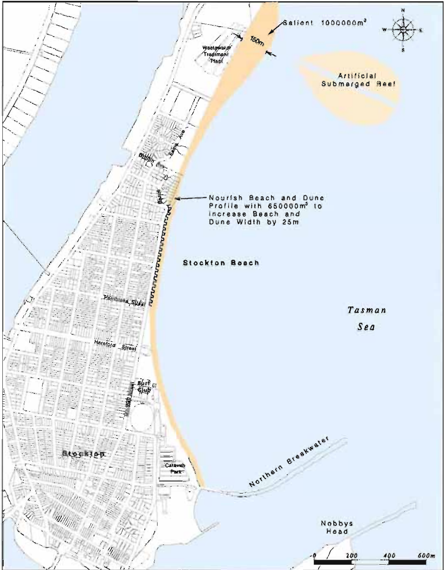
FIGURE 8.5 Conceptual Design of Artificial Submerged Reef
