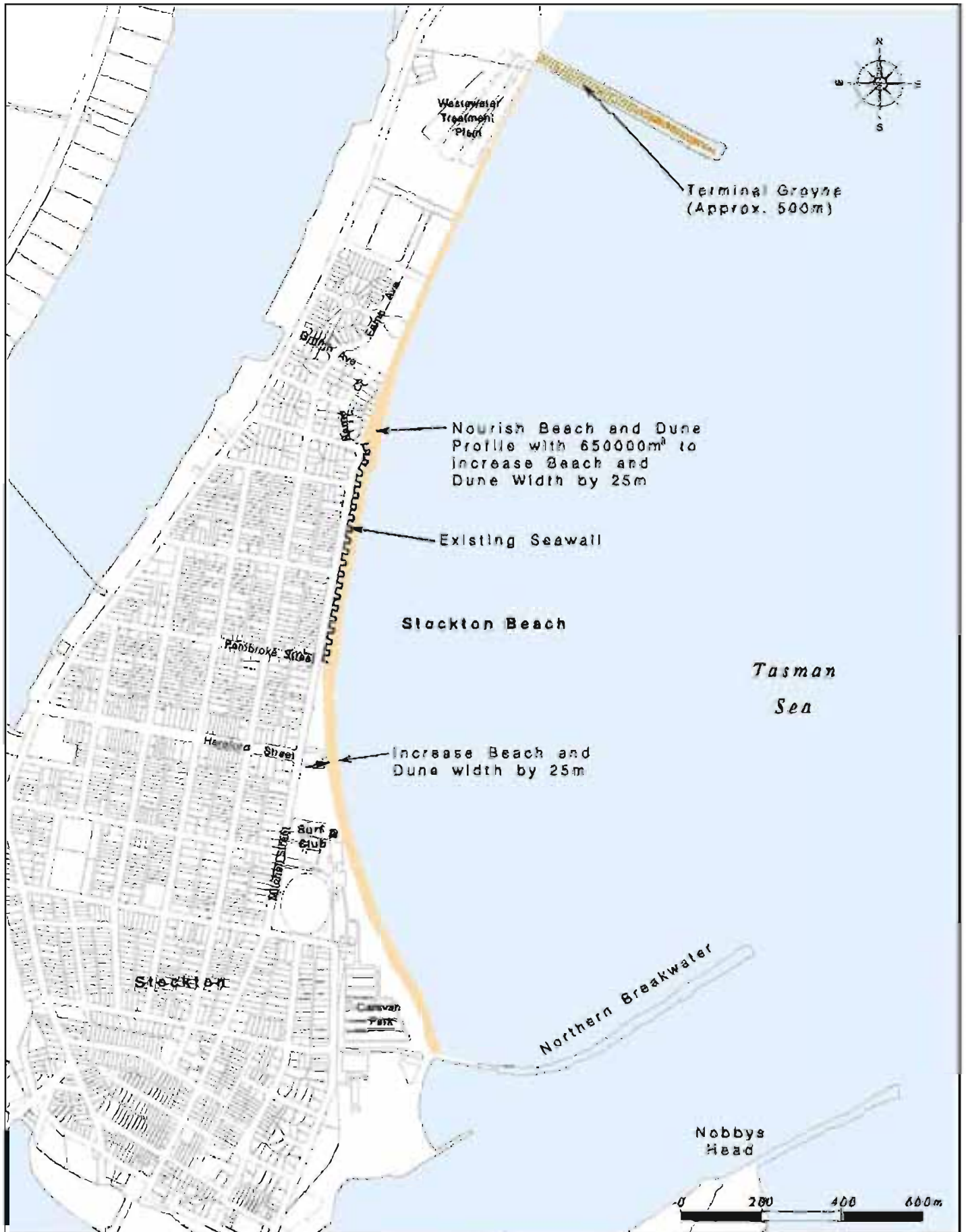
FIGURE 8.1 Terminal Groyne / Headland with Sand Nourishment Stockton Beach
