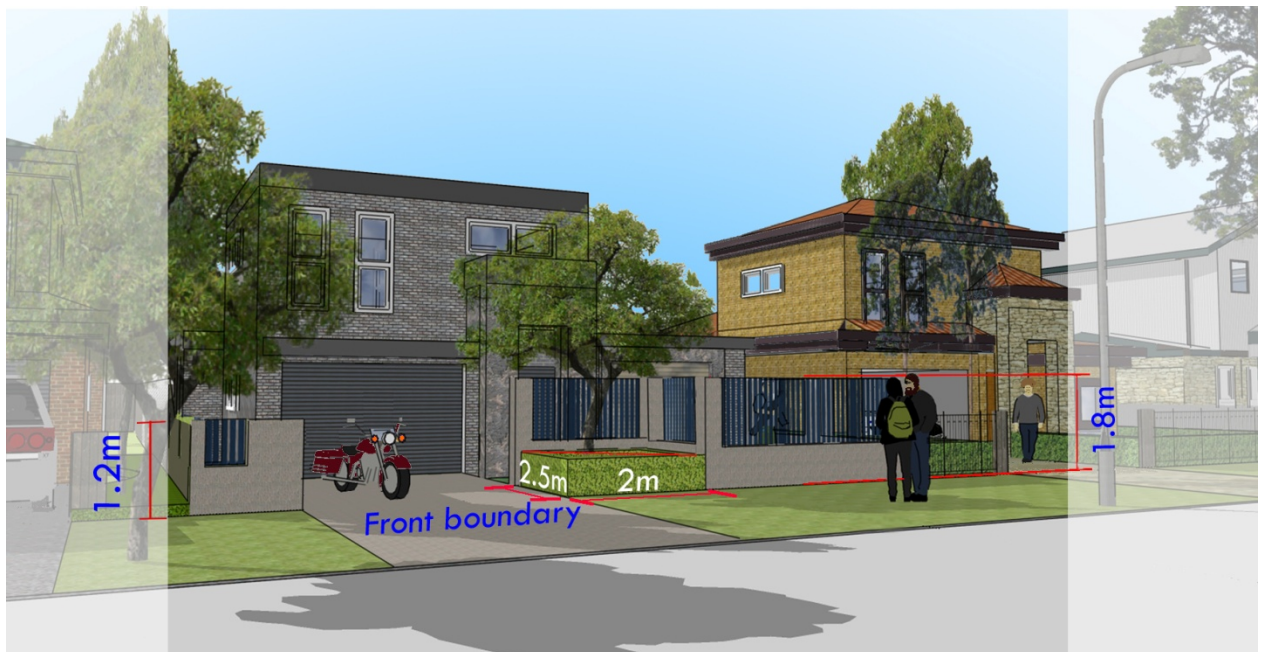
Figure 13: An example of a 1.8m transparent fence with landscaping complying with the driveway splay.
