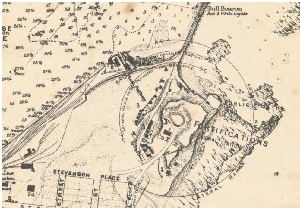
Figure 3.17. Detail from an 1887 harbourmasters plan of Newcastle showing Fort Scratchley, with the positions of the guns and their lateral range; a well-defined road leads to the site (Capt FW Sidney, RN, Plan of the Port of Newcastle, 1887, MAP RM 1588: http://nla.gov.au/nla.map-rm1588 )
