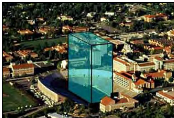
Illustration of the volume of stormwater captured by a single 50mm storm event in the City of Boulder USA
