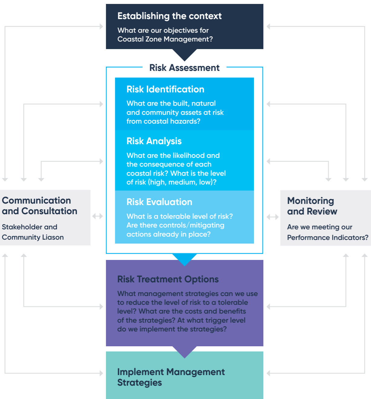
Figure 59: Risk management framework adapted to coastal zone management (BMT WBM, 2014(b) p36).
