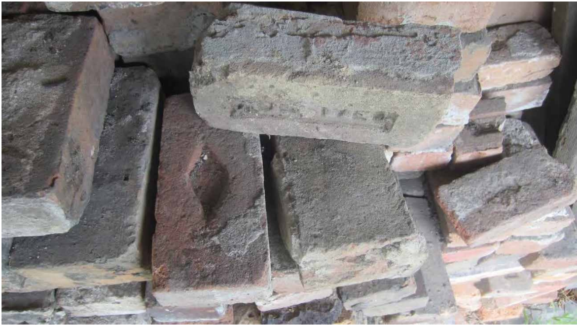
Figure 166. Brick stockpile, showing diamond pattern ( may be from original element of the house, clamp-kiln fired on site from local clay, c. 1849) and Gulliver frogmarks; Gulliver had a brickyard at the Glebe, Merewether; his activities are thought to have ceased in the early 1890s.
